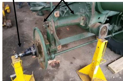
Later axle assembly Original axle assembly, showing shortened axle shaft
